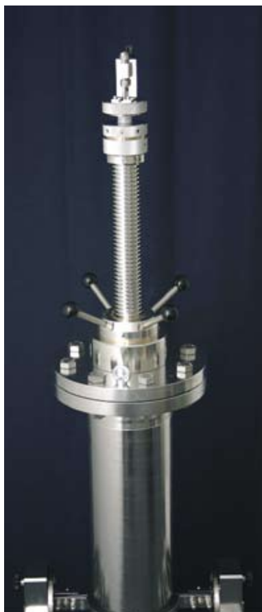
Column head of a stainless steel 100 x 1000 mm column, 50 bar, with swivelling column body.
