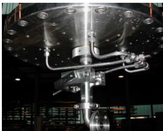
Ø 600 mm column, slurry outlet with separate tap, quadruple eluent outlet.
