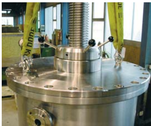
Ø 600 mm column as a special reactor for coating processes. Integrated level indicators assist assembly / disassembly for maintenance purposes.
