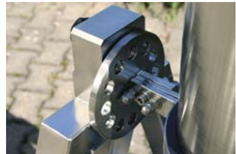
Notched wheels to fix a rotating column body.
